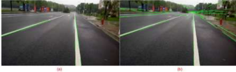
Fig 6. Comparison of the results of Hough transform in the detection of lines
